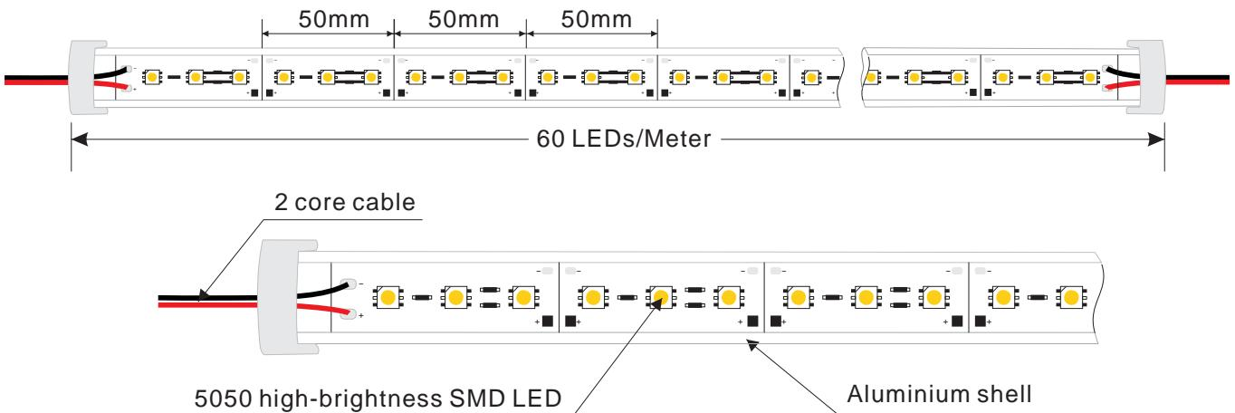
These strips are widely used in shop and bar illumination, it works at 12 DC, with super bright SMD LEDs, wide view angle, compact size, easy to install, Aluminium PCB holder help you to fix easily. Water-proof, long life span(more than 50000 hours)
