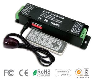
DN-DMX850DMX-PWM Decoder works to convert universal DMX512 digital signal to PWM signal, Which controlled by DMX512 console, with 8bit gray scale output per channel. Realize 0-100% brightness and various changing effect. And can control single color, RGB LED lights.
